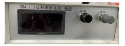
2. The reflectivity of white target in LDROBOT laboratory is 80.6%; that of the black target is 4.1%.
