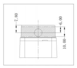
Other mounting dimensions are shown in the following diagram with a tolerance of  $\pm 0.2$  (in mm):
