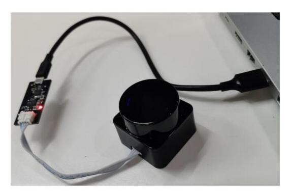
3. Place it in the test environment and click the start button of the upper computer to present the scan results, as shown in the picture below:
