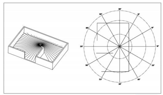
The product is mainly suitable for the navigation and obstacle avoidance of robots (e.g. floor mopping robots and service robots) by performing a  $360^{\circ}$  scan of the indoor layout and building a map so that a walking path can be planned. It is also suitable for robotics education and research, etc.
